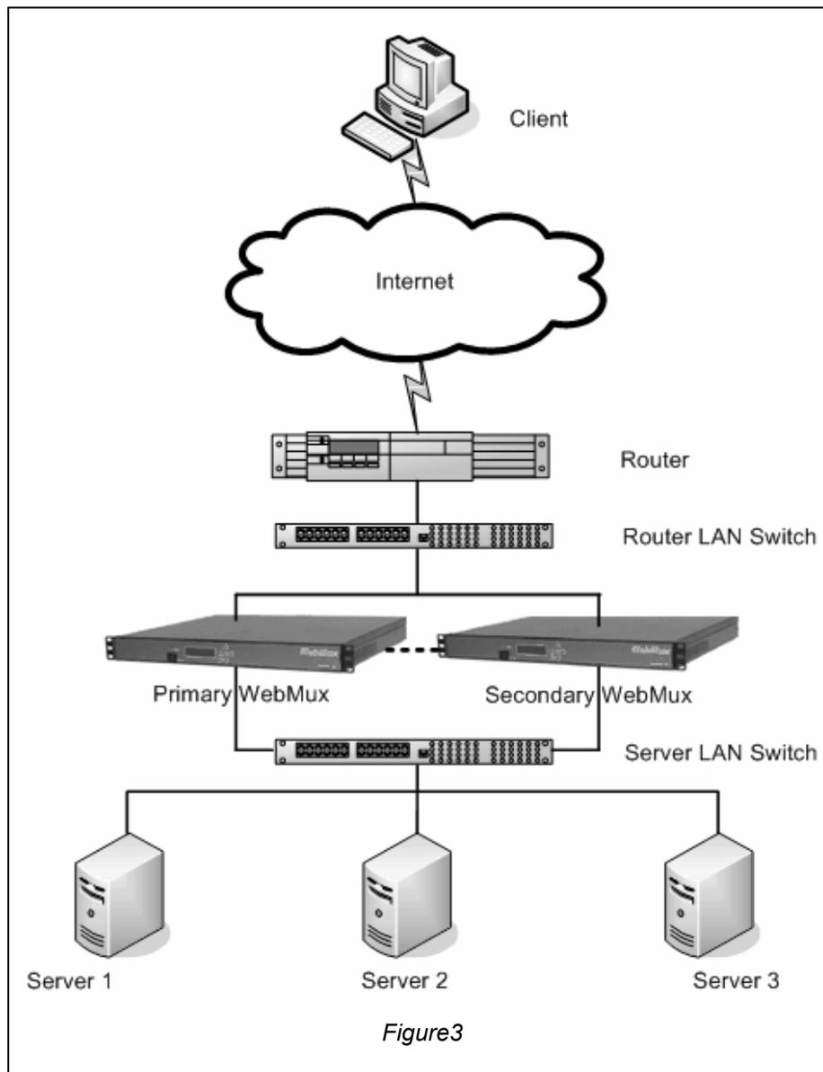
A government agency in Sydney, Australia, uses paired WebMuxes spread out over distance between two campuses, with one WebMux and an identical server farm located at each campus. This configuration additionally provides protection against local environmental disasters, since if one campus goes offline the other automatically takes up the workload.
