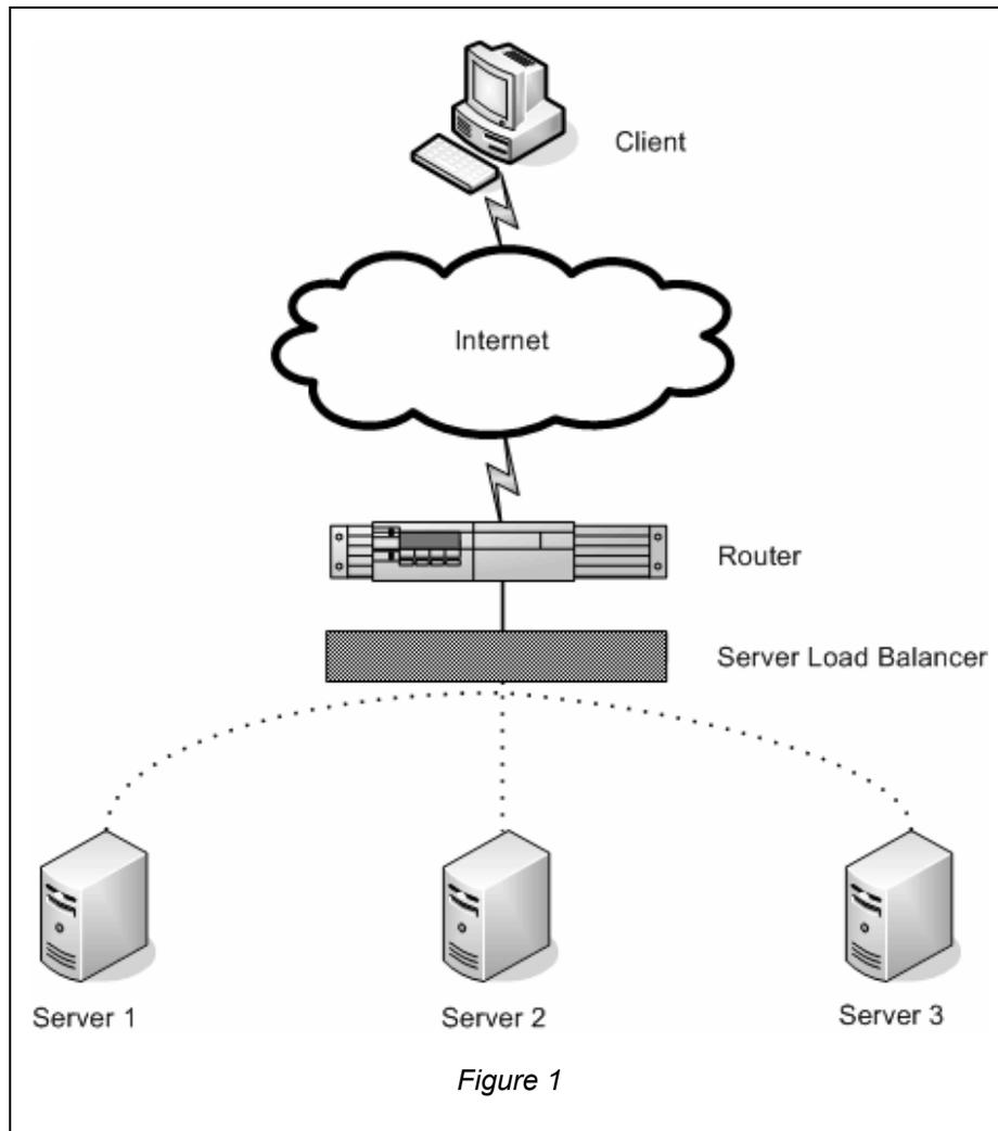
bogged down servicing certain transactions. More sophisticated allocation algorithms take into account real-time performance characteristics, such that the least busy servers can be sent more traffic. Some algorithms allow the allocation to be skewed based on the inherent performance characteristics of the servers, so that more powerful servers are allocated a heavier load.
