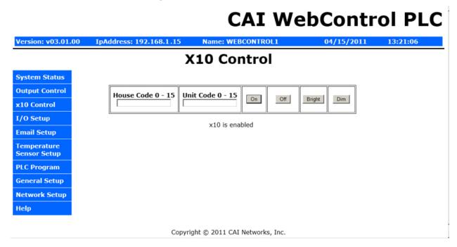
Please note the Bright and Dim function only working for X10 Lamp Module. Each time a Bright or Dim command sending out, only the last On/Off device in the same house code range being addressed, due to X10 RF spec.
