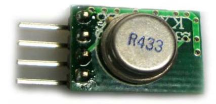
This kind of RF transmitter normally has Ground, +POWER, and DATA pin. Connects the +POWER to TTL output pin 7, and DATA to the TTL output 8, and the Ground to TTL block number 9 or 10. Please note, do NOT use TTL7 to power any other device, over current on TTL7 will cause permenant damage to WebControl and its not covered by warranty.
